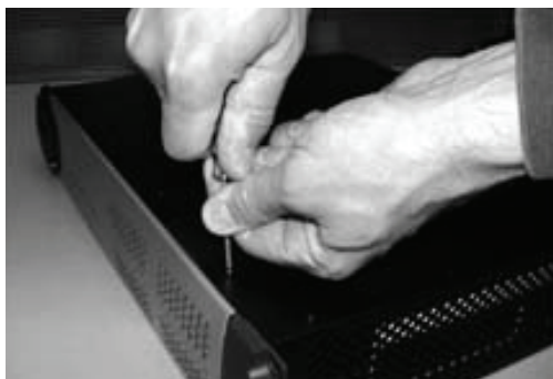
Removing the top cover screws
